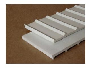
Attributes: Low stretch, stable belt made from RAV compound which is a blend of PVC and NBR Rubber. FDA grade white belt with a meat cleat profile for incline conveying. Good resistance to various oil, grease and cleaning solutions.
