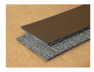
Attributes: Medium duty, general purpose conveyor belt used on many belting systems. Interwoven carcass plus brushed clean bottom surface for lower coefficient of friction. High strength, tear resistance, low stretch.
