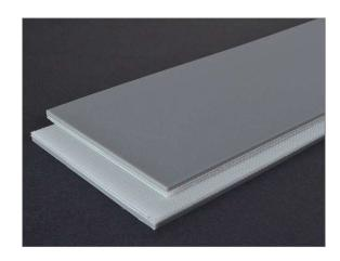
Features: 3-1600 belt features a low durometer PVC top cover providing a "sticky" carrying surface. This belt has a 2 ply monofilament carcass and can travel at high speeds with low noise. It is also known as a 'Sticky Top' belt, is cross rigid, and nonmarking.
