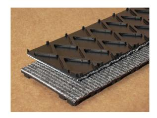
Attributes: Interwoven polyester carcas with a 1/8" raised Z profile. Belt has an oil resistant PVC compound. Z-Cleat must be recessed for lacing. OAG includes profile, use recessed OAG for lacing recommendation.
