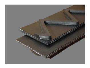
**Attributes:** Belt features a 1/4" high interconnected Z Profile. Heavy duty 2 ply interwoven belt. Thickness without the profile is .220.
