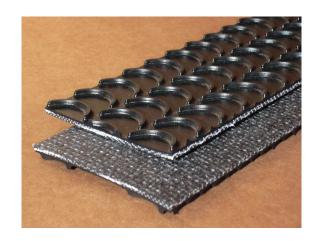
Attributes: Features an interwoven carcass with a 1/8" high half moon crescent impression. Belt has a brushed bottom for a low coefficient of friction and oil resistant PVC compound. Also available in white and in heavier gauges.
