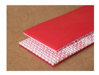
Attributes: Tough, abrasive, red urethane belt. Interwoven polyester reinforcement with friction surface bottom. Urethane top resists cutting and abrasion from metal, glass and abrasives.
