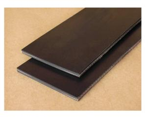
Attributes: Static conductive, moderately oil resistant, fire retardant and MSHA approved for grain elevators. 5-2335 belt is not approved for use in underground applications.
