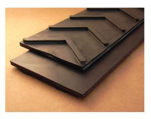
**Attributes:** 1/4" high x 6" wide chevron profiles available staggered across belt. Reinforced MOR belt for heavy duty incline with moderate oil resistance.
