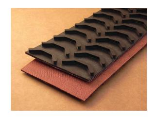
Attributes: Features 3/16" high by 1-3/4" wide mini bucket profiles in a staggered pattern. Cleats are spaced on 2" centers across the belt and 1" centers down. Bottom surface is bare.
