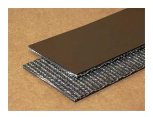
Attributes: Popular general purpose belt with interwoven carcass and smooth PVC top cover. Bottom cover is brushed clean to lower the coefficient of friction. High strength, low stretch belt.
